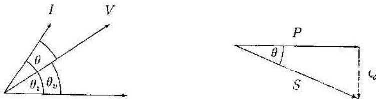
FIGURE 2.4 Phasor diagram and power triangle for a capacitive load (leading PF).
